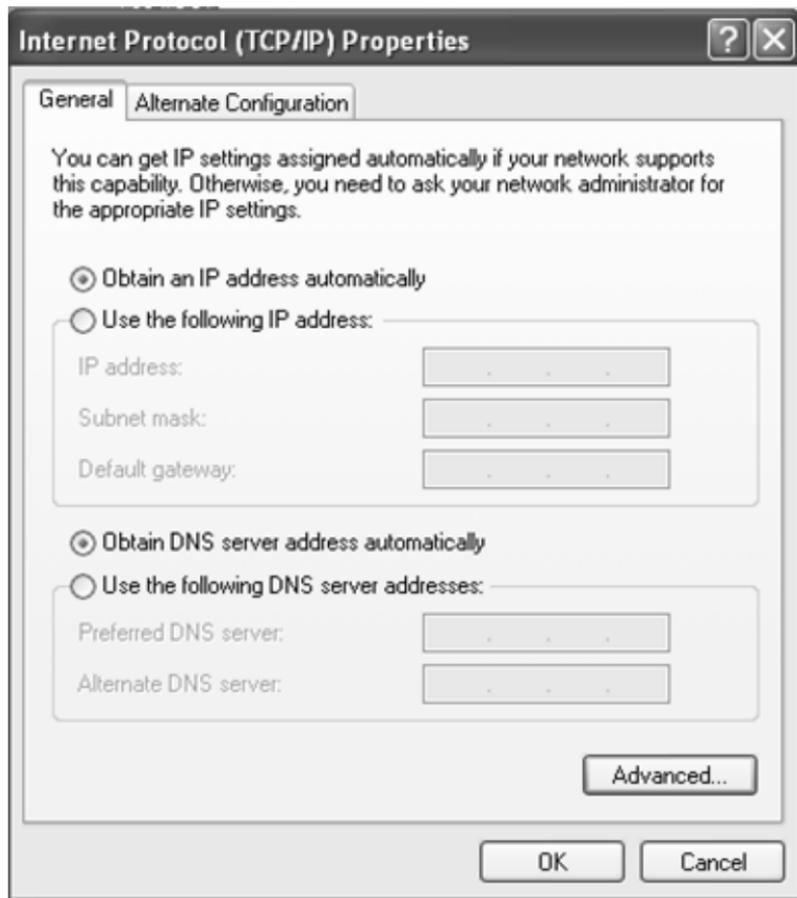
Figure 4 IP and DNS configuration
